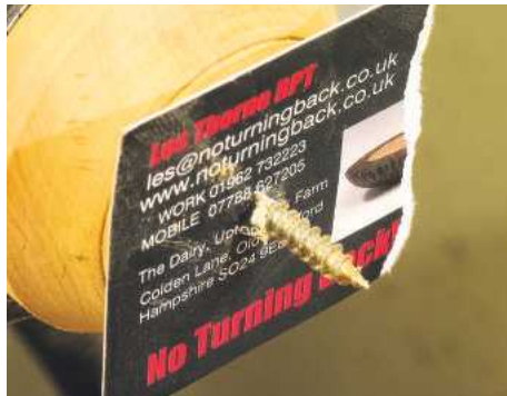
▲ Pic.10 After you have sanded the top turn the apple around onto the screw chuck; protect the finished part of the apple with a business card
